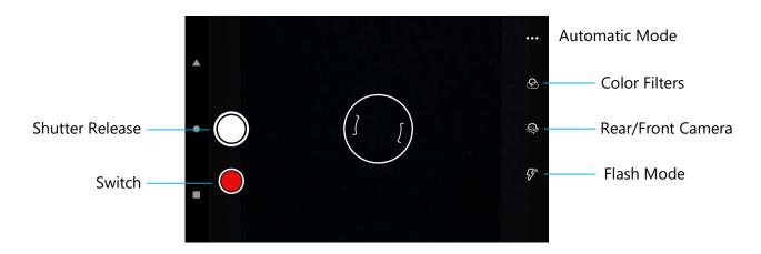
**Switch** – A switch for Video Capture mode.
