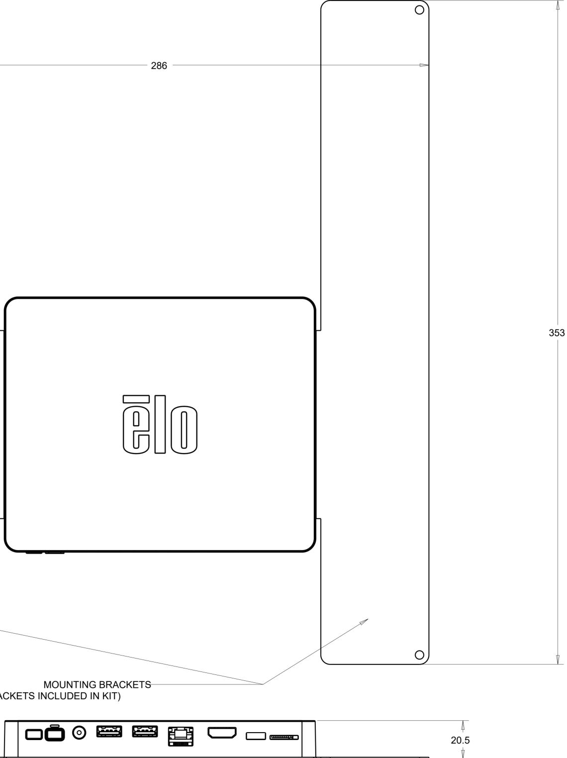
DIMENSIONS ARE IN MILLIMETERS
