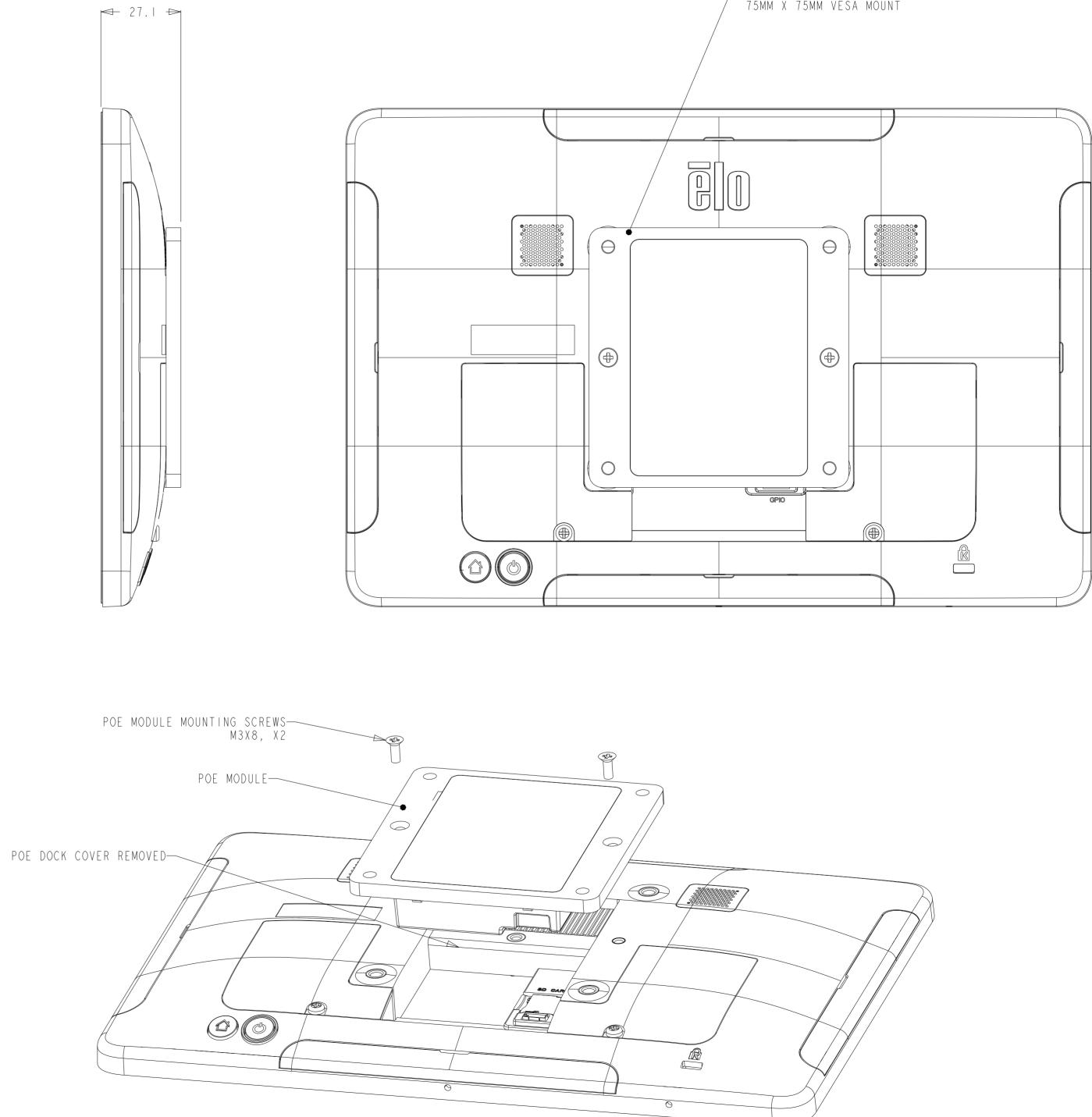
POE MODULE INSTALLED INCLUDES THROUGH HOLES FOR 75MM X 75MM VESA MOUNT
