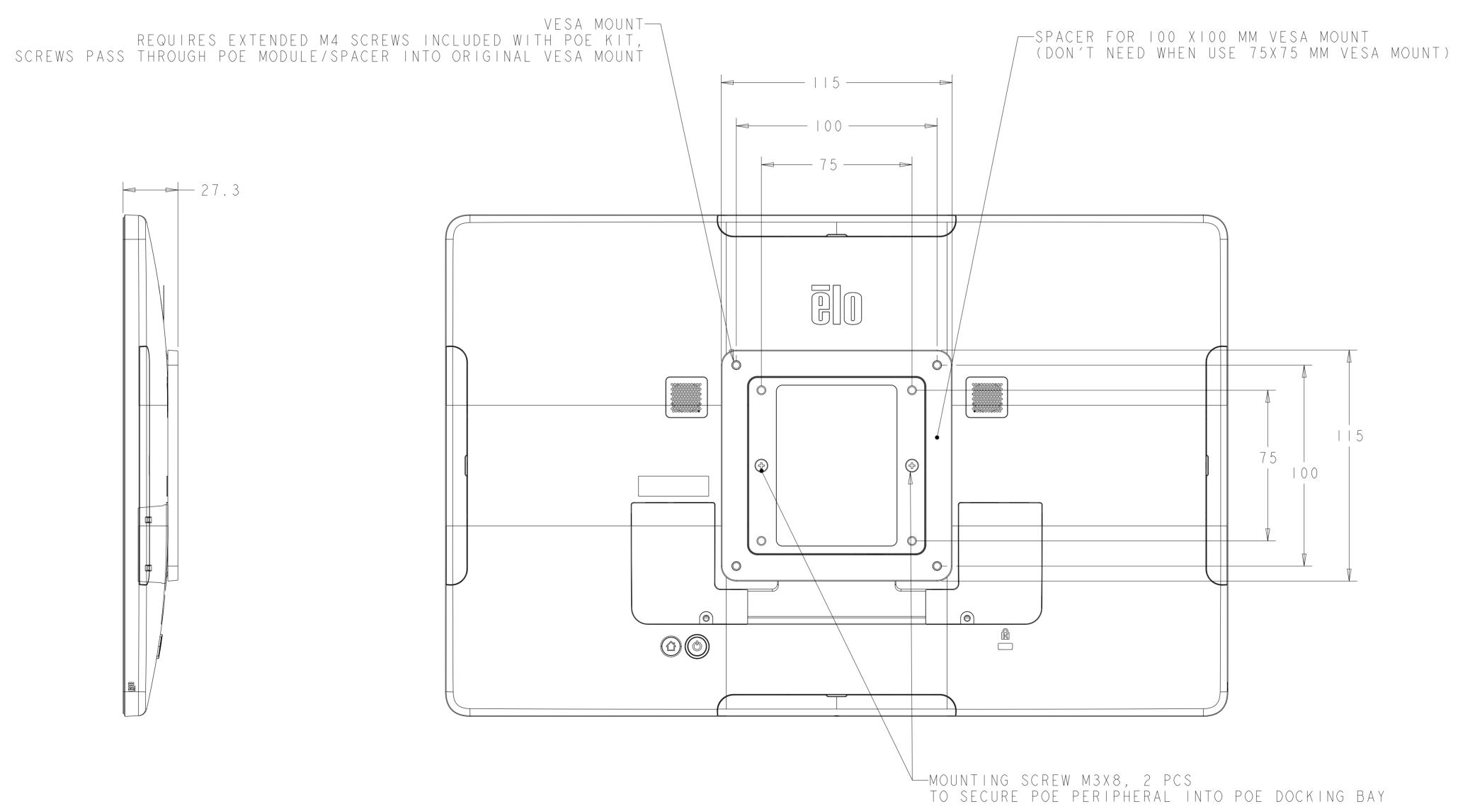
POWER OVER ETHERNET (POE) ADAPTER KIT P/N: E4I3396 (OPTIONAL KIT, PURCHASED SEPARATELY) POE COVER REMOVED AND POE PERIPHERAL INSTALLED
