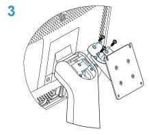
Add the display bracket to the stand using (3) screws from bag A.
