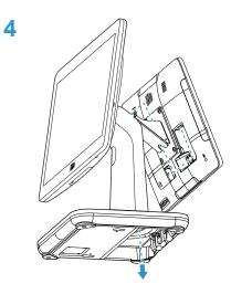
Attach a monitor to the display bracket using (4) screws from bag B. Plug in the USB-C cable and route through the stand.
