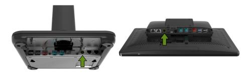
**3** Make additional connections from the bottom of the stand module or the Touchcomputer.
