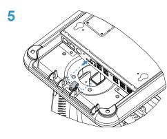
Plug in the other end of the USB-C cable to the base and secure with the supplied cable clamp and screw from bag C.
