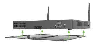
3. Mount bracket to table using four M4 or #8 mounting screws (not included) Screw type depends on table construction. The screw head height must be 3.0mm (0.118") or less.
