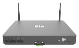
6. Connect a display with HDMI or USB-C, connect the power supply, and WiFi antennas (if WiFi is required) Press the power button to power up the computer and proceed to registering Windows. Refer to user manual for detailed setup instructions.
