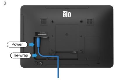
Connect the power cable. The system will power on automatically when plugged in. A tie-wrap (included) can be used to secure the power cable from accidental removal.
