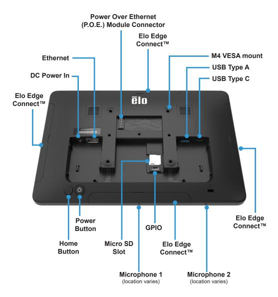
Maximum Torque for M4 VESA mount screws = Hand tighten only (Max. 12.4 in-lb/1.4N-m)
