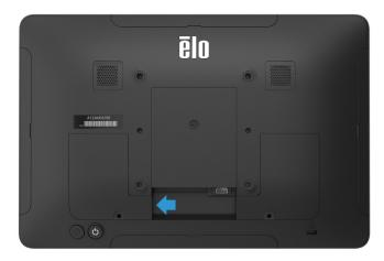
Remove the left side cable cover by lifting upward
