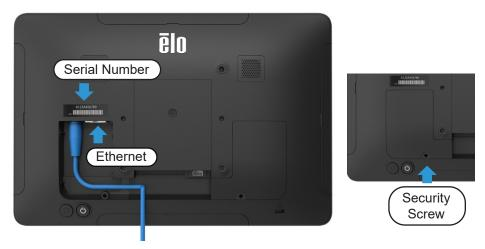
Connect an Ethernet cable now (or setup WiFi later). Once all cables are connected, reinstall the cable over and secure with included security screw.
