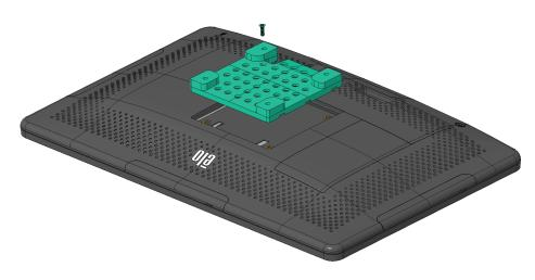
2. Assemble adaptor to I-series using (4) M4 flat head screws (included with kit), in 75mm VESA mounting holes.
