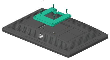
3. Assemble desktop stand to I-series using (4) M4 pan head screws included with stand.
