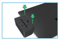
4.Install the 2 flat head screws included with the kit.
