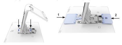
**3** Remove the cable cover door and route the USB-C cable from the I-Series 4 Slate Display under the stand opening and connect to the USB-C port on the rear of the display.
