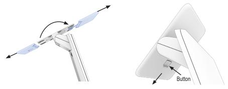
2 Secure the I-Series 4 Slate Display to the stand by installing the M4x6 flat-head screws (4 included with stand kit) through the mounting plate and into the back of the display. Do not use longer or shorter screws. Slide the plastic top cover over the mounting plate making sure the cover sits against the rear of the display. Then slide the lower cover up until the button snaps in place.
