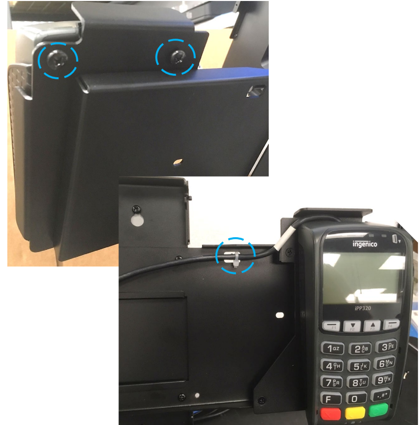
Add screws from bag "J"; do not over tighten. Add zip-tie.
