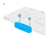
Gently insert the speaker bar kit into the peripheral bay taking care to ensure the connector mates properly.
