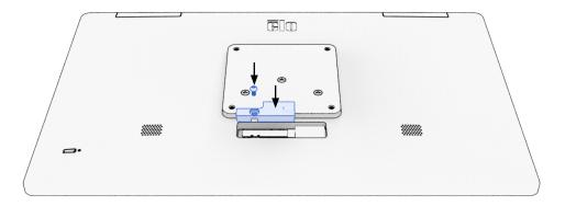
**2** Plug the USB-C cable from the I/O Hub into the rear of the Slate display.
