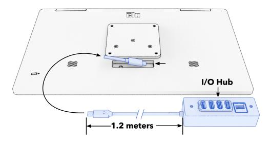
**4** The Slate display has four mounting holes on the rear. The I/O Hub has two mounting holes which allow it to be mounted out of sight. See dimensional drawing for mounting hole details.
