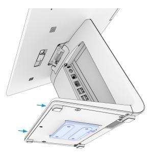
**5** Secure the system to the bracket using the screw included in the accessory box.
