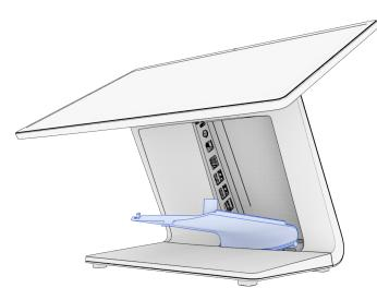
**2** Route the DC power cable through the hole in the bottom of the stand and connect it as shown. Connect other I/O cables as needed (see back page). Make sure all cables route behind the plastic clip at the bottom.
