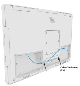
4 Reinstall the cable covers by snapping into the display and tightening the two screws. Mount on stand or wall using 75mm VESA mounting interface (15.6" model) or 100mm VESA mounting interface (other models) using included M4x12 screws. Press the power button to turn on the Touchcomputer.
