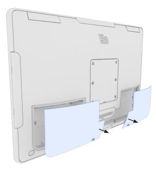
2 Connect the power adapter. Make additional connections as needed. Connect Edge Connect peripherals to edge Micro USB ports by removing covers as shown.
