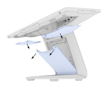
2 Connect the power adapter. Make additional connections as needed. Connect Edge Connect peripherals to edge Micro USB ports by removing covers as shown.
