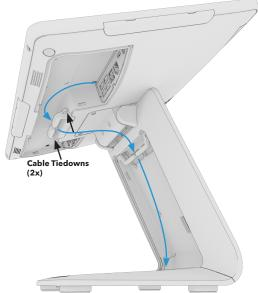
4 Reinstall the stand door by snapping into the stand and installing the two screws from step 1. Reinstall the cable covers by snapping into the display and tightening the two screws. Press the power button to turn on the Touchcomputer.
