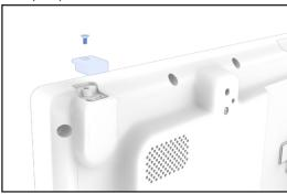
2. Connect Wi-Fi adapter, place large security cover over adapter and reinstall screw. (Large security cover included with Wi-Fi adapter kit)
