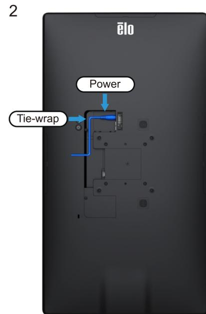
Connect the power cable. The system will power on automatically when plugged in. A tie-wrap (included) can be used to secure the power cable from accidental removal.
