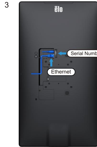
Connect an Ethernet cable now (or setup WiFi later). Once all cables are reconnected, reinstall the cable over and secure with included security screw.
