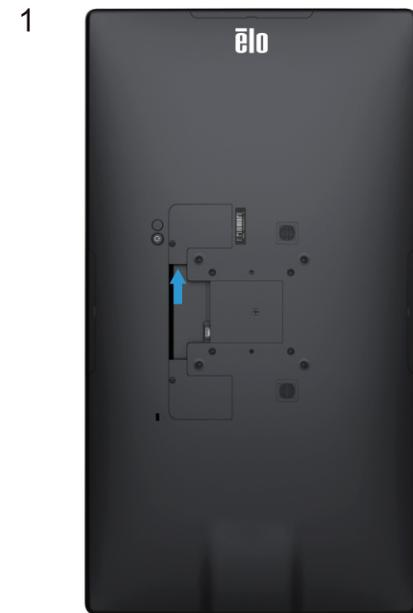
Remove the top side cable cover by lifting upward.
