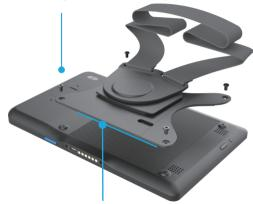
Align the straight edge of the shoulder strap bracket to the bottom/connector side of M100.
