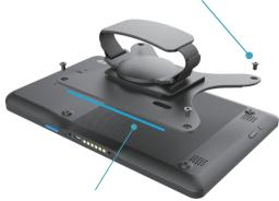
Align the straight edge of the rotating hand strap bracket to the bottom/connector side of Elo Pay M100.
