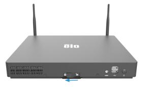
6. Connect a display with HDMI or USB-C and WiFi antennas (if Wi-Fi is required). Connect the power cable with locking thumbscrew. Press the power button to power up the computer and proceed to registering Windows. Refer to user manual for detailed setup instructions.
