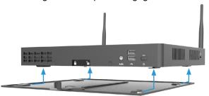
5. Slide the latch to the left to lock the computer onto the mounting bracket.
