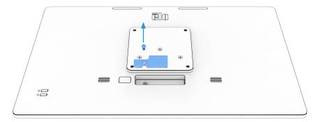
2 Plug the USB-C cable from the I/O hub to the rear of the I-Series 5 Slate display. The I/O hub has two threaded mounting holes which allow it to be mounted out of site if desired. See dimensional drawing for mounting hole details.
