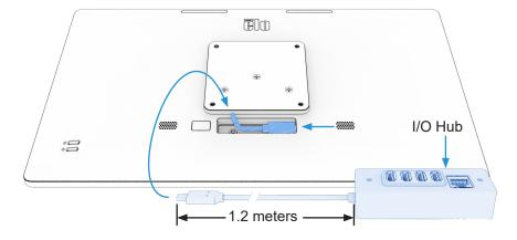
**3** Reinstall the cable locking screw and bracket on the rear of the I-Series 5 Slate display. The bracket slides in at an angle and has two small hooks that engage with slots inside the cable cavity. The bracket must be secured with the included screw.
