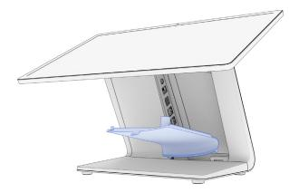
2 Route the DC power cable through the hole in the bottom of the stand and connect it as shown. Connect other I/O cables as needed (see back page). Make sure all cables route behind the plastic clip at the bottom.
