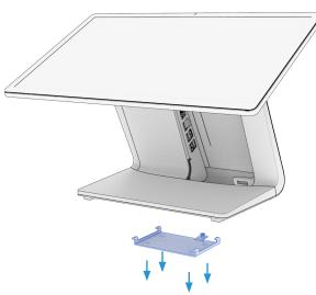
4 Lower the system onto the bracket and slide it back, ensuring the bracket hooks engage with the slots on the bottom of the system.
