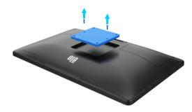
2 Assemble adaptor to I-series using (4) M4 flat head screws(included with kit), in 75mm VESA mounting holes.
