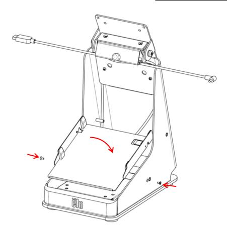
**4** - Re-assemble printer tray using (2) screws, L & R side.
