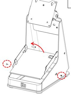
**1**- Remove (2) screws (L & R side) and pull-out printer tray. Keep screws for reassembly.
