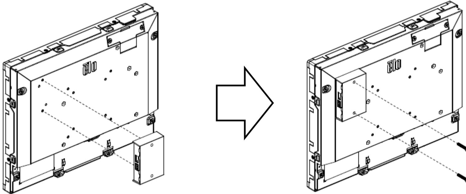
2. Please connect the cable from power source to convertor via terminal block for 24V input and plug 12V DC jack to our monitor for 12V output.
