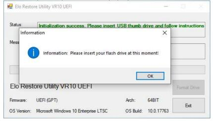
4. After the flash drive is inserted, you shall see a window as shown below. Click "Format Drive" to continue the process. PLEASE NOTE THAT ALL DATA WILL BE LOST DURING THIS PROCESS.
