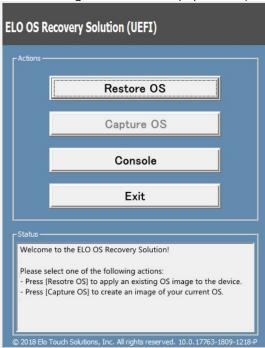
5. Select **Restore OS**. The system will test your hardware automatically. Once the process completes, click **Start** button to perform the system recovery function.
