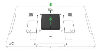
Install optional spacer included if using 100x100mm VESA mount. Place it over the adaptor before adding VESA mounting bracket.
