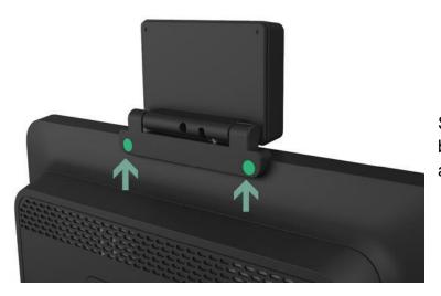
Step 5: Attach the screws in the accessory bag to protect the mera and adjust the angle as needed.
