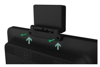
Step 4: Install the two screws of the accessory bag.
