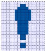
If the temperature exceeds 60 °C, the following icon will appear in the Main Menu. This will indicate that the Thermal Protection Mode is active. If the display internal temperature is not reduced below 65 °C for 5 minutes, the display will automatically turn off 60 seconds to prevent permanent damage.
