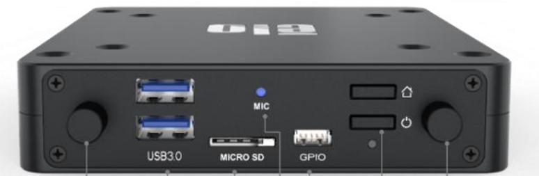
ANNTENA Covered by Rubber Cap    USB 3.0 X2    SD Card    GPIO    Power + Home Button    ANNTENA Covered by Rubber Cap
