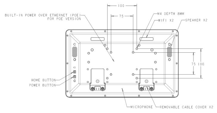
For the 22inch size, A four-hole 75x75 mm and 100x100 mm mounting patterns for M4\*6 screws are available. The VESA FDMI-compliant mounting is coded: VESA MIS-D, 75,C and VESA MIS-D, 100,C
