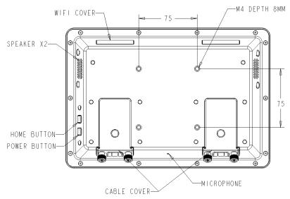
For the 15inch size, A four-hole 75x75 mm and 100x100 mm mounting patterns for M4\*6 screws are available. The VESA FDMI-compliant mounting is
