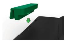
Gently press the MSR into the peripheral bay making sure the connector is mated.
