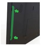
Remove the selected peripheral cover from the display head to expose the peripheral bay.
