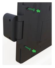
Install the 2 flat head screws included with the kit.
