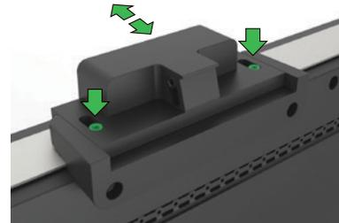
Adjust the forward/back position of the webcam by loosening the two highlighted screws with the included 3mm allen wrench and sliding the webcam head forward as needed. Tighten screws when done.
