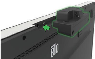
Gently insert the webcam into the peripheral bay taking care to ensure the connector mates properly.
