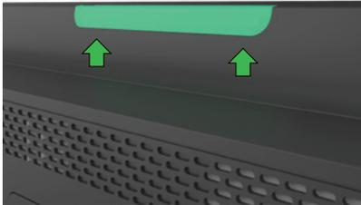
Remove the selected peripheral cover from the IDS Display.
