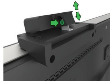
Adjust the tilt angle of the webcam by loosening the highlighted screw and lifting up on the back of the webcam head. Tighten screw when done.
