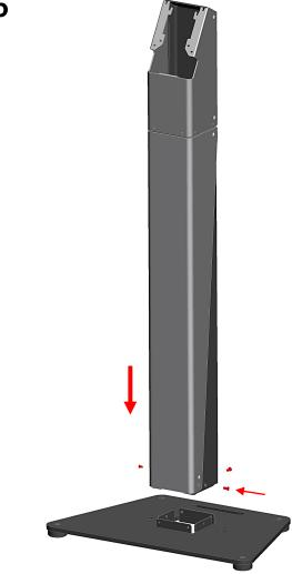
Assemble base plate to tower using (4) screws from bag "K".
