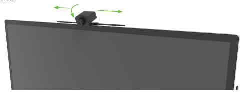
**Option 2**: Choose the left or right side location for smaller or narrow meeting rooms or where participants are located close to the camera. After installation, users can slide the position up or down and tilt toward the center of the IDS Display to center the camera viewing area at eye level allowing for a more face to face conferencing experience.
