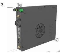
Use a screw driver to tighten the ECM security screw (hand tight only). The security screw must be installed to ensure the ECM does not come out inadvertantly.
