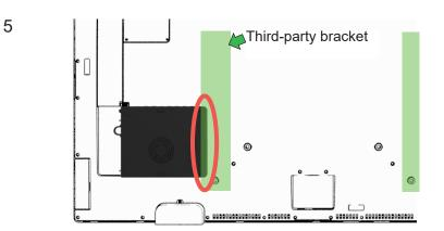
Some third-party VESA mounting systems may interfere with installation or removal of the ECM. The ECM kit includes a set of 15mm spacers, 35mm spacers, and longer mounting screws to aid in adding additional clearance between the VESA mount and the ECM. Additional screw lengths (not included) may be required depending on the mounting system. Do not block any air venting on the ECM or IDS display.
