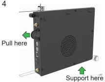
To remove the ECM, power down the system and loosen the security screw.
