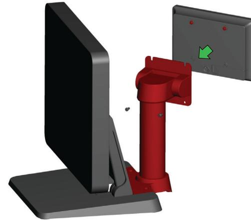
Partially install (2) M4x8mm screws on top of monitor leaving gap to hang monitor on slots of mount plate. Install the other (2) M4x8mm screws on bottom of monitor and tighten all 4 screws.
