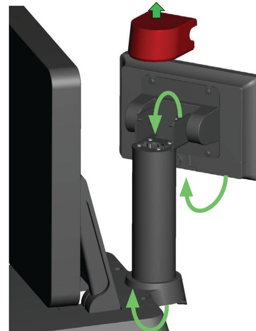
Remove pole hinge cover and route cables through pole and connect to computer. Reinstall pole cover.
