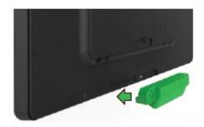
Gently insert the bar code scanner into the peripheral bay taking care to ensure the connector mates properly.
