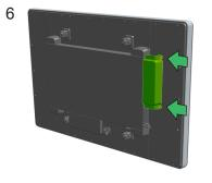
Install security cover by tightening the two thumbscrews into the top and bottom cover brackets
