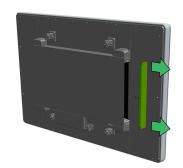
Remove the two cover plate screws and pull the cover plate out.
