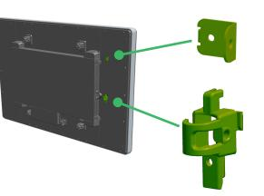
Install the top cover bracket using M3 screw included in kit.
