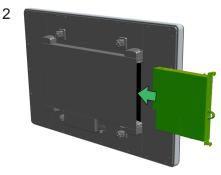
Slide the computer module into the opening until it stops.
