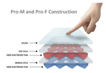
together with Optically Clear Adhesive (OCA). The conductive grids are printed onto thin PET film material.
