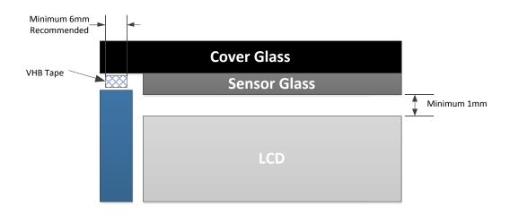
Figure 2-3. Standard Integration of a PCAP Touchscreen without Bezel (not to scale)
