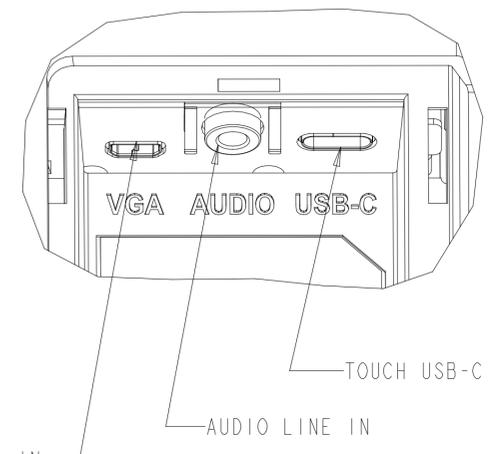
VGA IN (VGA-DB15-TO-MICRO) VGA-DB15 TO MICRO CABLE SOLD SEPARATELY
