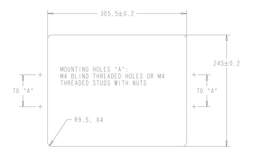
DIMENSIONS ARE IN MILLIMETERS
