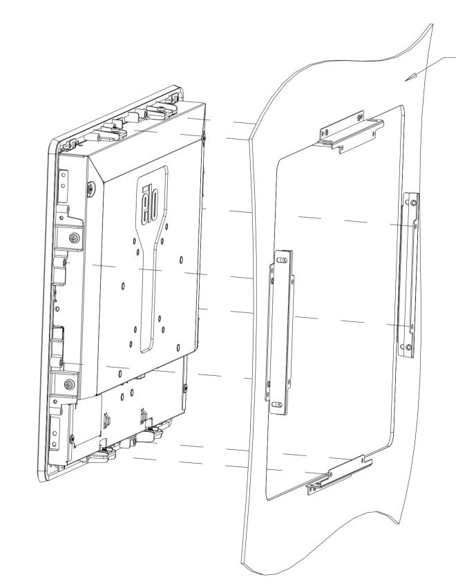
CUSTOMER PANEL (NOT INCLUDED) MIN THICKNESS = 3MM MAX THICKNESS = 12MM
