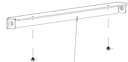
INSTALL BOTTOM BRACKET FIRST USING 2X M4 SCREWS (INCLUDED)
