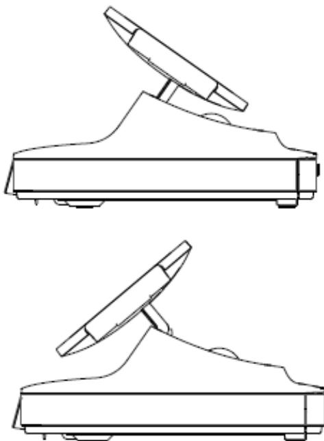
Figure 3. Elo PayPoint iPad® Dock display head can be flipped and supports two configurations:
