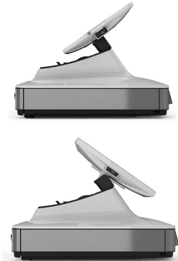
Figure 3. Elo PayPoint Plus display head can be flipped and supports two configurations: Elo PayPoint Plus register cashier-facing view (top) and customer-facing view (bottom)
