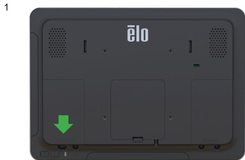
Remove the left side cable cover by sliding downward
