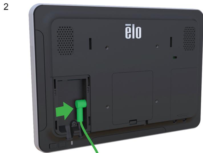
Connect the power cable. The system will power on automatically when plugged in.
