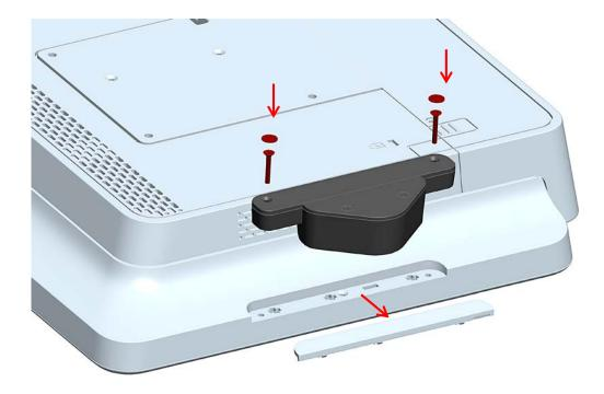
Remove cover from computer. Add i-button reader using 2 screws provided. Add 2 mylar covers provided on top of screws.
